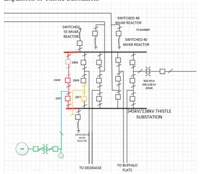
In addition to the identified Network Upgrades, there are specific Interconnection Facilities which ITCGP will construct, own, operate, and maintain. These facilities include the new line entrance structure and 345kV disconnect switch on the end of the radial line at the ITCGP switching station as well as any ITCGP relaying and control equipment required for the protection of the developer's radial line.
